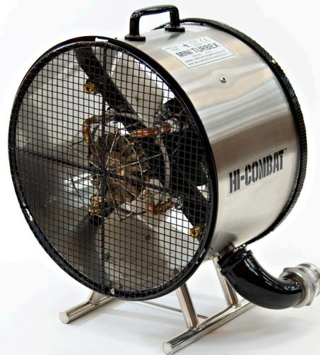
Angus **HI-COMBAT** Mini-Turbex unit is a rapid deployment, first aid high expansion foam generator which produces up to 100 cubic metres (3,500 cu.ft) of foam bubbles per minute. This **HI-COMBAT** Mini-Turbex is capable of producing expansion ratios between 260-360:1. With special re-inforced smoke ducting, it can also be used for rapid smoke extraction (SX), positive pressure ventilation and removal of foam once the fire is extinguished.
