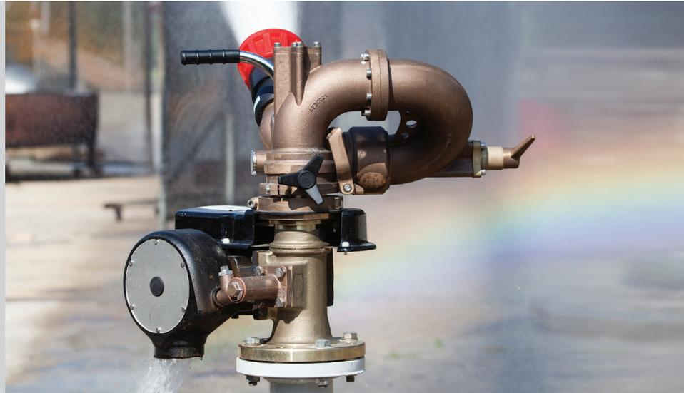
The Angus OM-80 is a nominal 80mm waterway Oscillating Monitor, designed to provide optimised hydraulic efficiency and long throw performance when the Angus Long Throw (LTN) nozzles or (LTC) cannons are fitted. The compact low profile configuration, makes this monitor particularly suitable for installation on towers, aircraft hangars, offshore platforms for helideck protection and other areas where space is limited.
