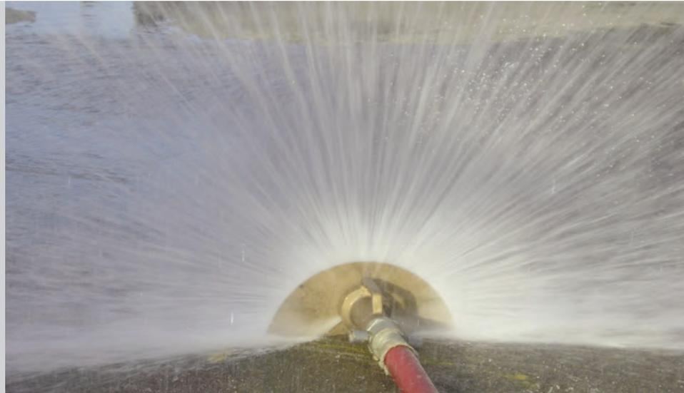
The Angus Fire HYDROshield directs the flow of water into a flat fan shape. The fan, or water curtain, is used to protect fire fighters from smoke, flame, radiant heat and to stop the flow of gases at ground level.
