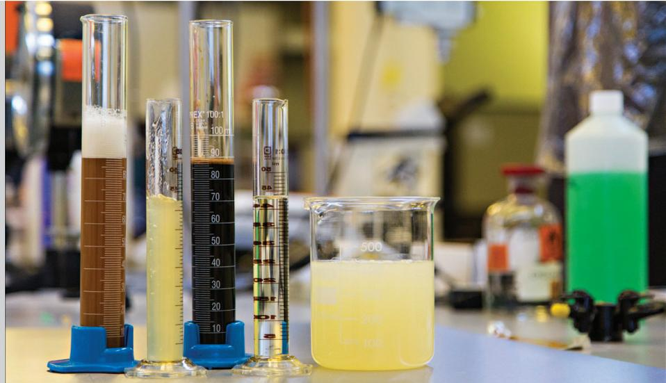
Firefighting foam concentrates are the preferred extinguishing medium for many flammable liquid risks. It is vital the foam performs when called upon during any stage of its operational life, therefore it is vital that the foam is tested regularly.
