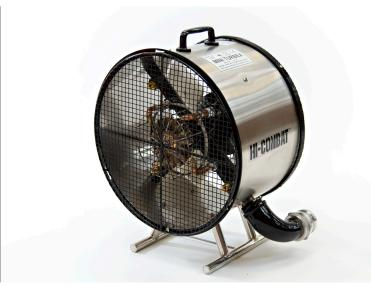
Angus **HI-COMBAT** Mini-Turbex unit is a rapid deployment, first aid high expansion foam generator which produces up to 100 cubic metres (3,500 cu.ft) of foam bubbles per minute. This **HI-COMBAT** Mini-Turbex is capable of producing expansion ratios between 260-360:1. With special re-inforced smoke ducting, it can also be used for rapid smoke extraction (SX), positive pressure ventilation and removal of foam once the fire is extinguished.
