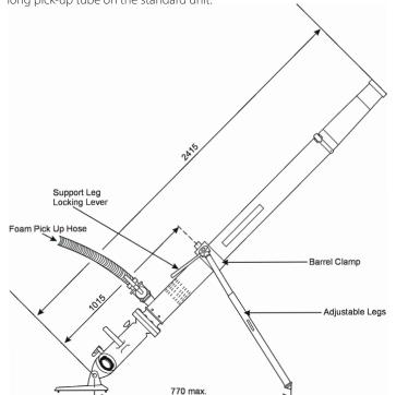
The solution throughput is 4,500 litres/ minute at 10 bar and the foam is expanded to 5:1. This low expansion gives maximum throw whilst ensuring a good quality foam blanket. A pressure gauge is provided to ensure maximum operating pressure are not exceeded.
