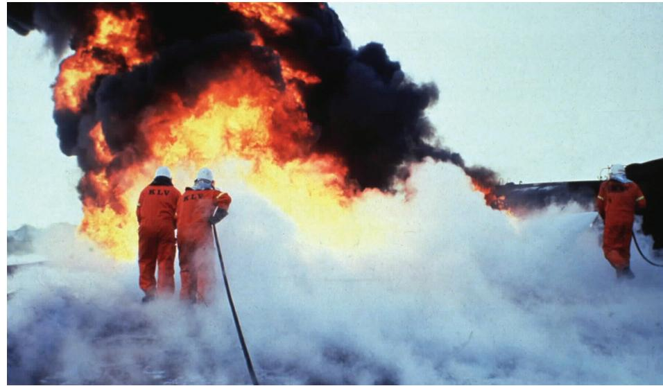
Petroseal<sup>C6</sup> 3 is a superior quality Film-Forming FluoroProtein (FFFP) fire fighting foam concentrate for extinguishing and securing flammable hydrocarbon liquid fires.
