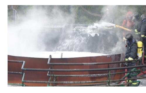
A fluorosurfactant free training foam which mimics the application and physical properties of Angus Tridol<sup>C6</sup> S AFFF 3% fire fighting foam.
