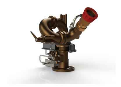
The Angus OM-80 is a nominal 80mm waterway Oscillating Monitor, designed to provide optimised hydraulic efficiency and long throw performance when the Angus Long Throw (LTN) nozzles or (LTC) cannons are fitted. The compact low profile configuration, makes this monitor particularly suitable for installation on towers, aircraft hangars, offshore platforms for helideck protection and other areas where space is limited.
