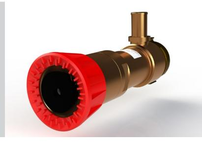
The LTN1900 - SI is a self-inducing foam nozzle for use on hydrocarbon fires with film forming foam like Petroseal or Tridol. It can be fitted to the Angus Streamline HM-80 and OM-80 monitors to provide a simple foam station.
