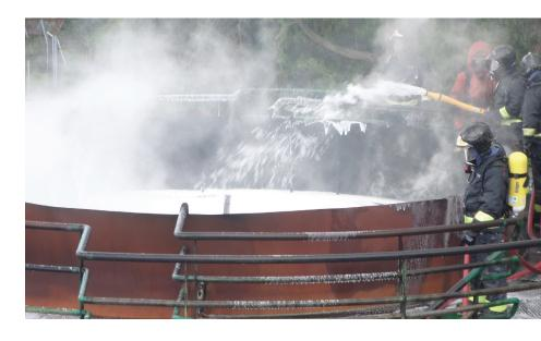
A fluorosurfactant free training foam which mimics the application and physical properties of Angus Petroseal<sup>C6</sup> 6% FFFP fire fighting foam.
