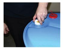
If you suspect that the venting bung assembly is not working then you should replace the venting bung with a new one and then fit a new tamper-evident seal to the filling neck.
