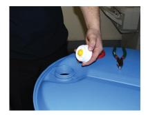
With the tamper-evident seal removed, unscrew the bung in an anti-clockwise direction. During its removal watch out for any slight release of gas pressure. The presence of a slight pressure or vacuum in the container or / and or an obvious blockage of the hole in the plastic shroud indicates that the venting bung assembly is not working as it should do to allow the container contents to 'breathe'.
