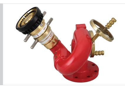
The Angus GMB48 fire monitor is a simple and reliable design with non-reversible worm and wheel gearbox control in both the horizontal and vertical plane. Movement is controlled by dual hand wheels.
