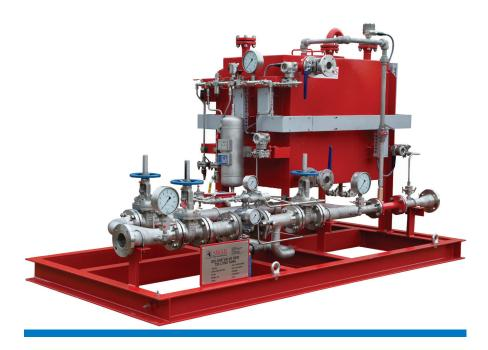
For LNG risks, Angus Fire can design and manufacture a fast acting foam proportioning system to mix the foam concentrate into the water supply. This can often be a complex bespoke system of foam skids and remote induction based on site requirements. Foam Induction systems fitted with In-Line Inductors or Balance Pressure Proportioning can be used depending on the specific design. Systems typically require 500:1 expansion, which means relatively small foam tanks can be specified.
